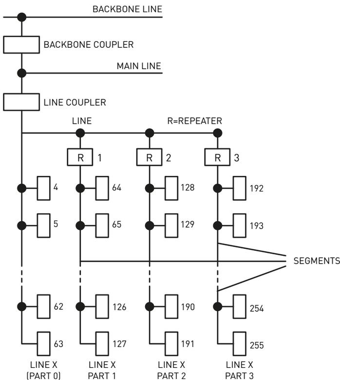
Fig.1. Connection of repeaters to a bus line
